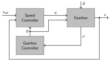
reference speed  $v_{ref}$  rotational speed  $\omega$
